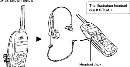
When the headset is connected to the handset, make sure to use the headset to talk with the caller. If you want to have a normal cordless phone conversation, disconnect the headset
